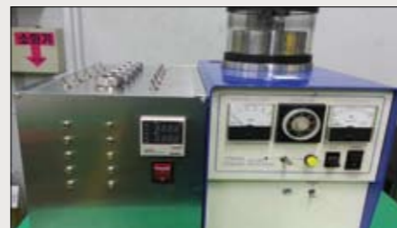
A prototype of OsO 4 coater for improving image data of nano-size sample
