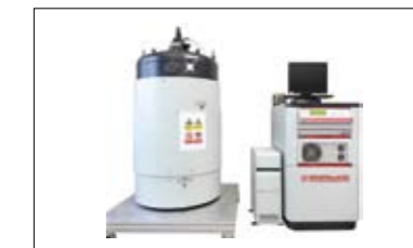
16 T Physical Property Measurement System
