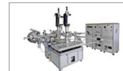
NAP-XPS analysis under pressure (up to 25 mbar) and humidities similar to those encountered in natural environments
