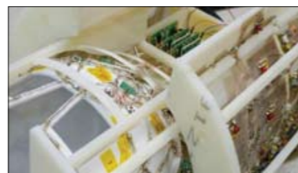
Multi-channel transmit/receive RF coil built, Tx/Rx = 8/32 channels, (image: CFMM, Ontario, Canada)
