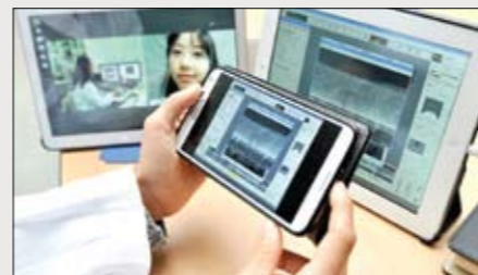
Real-time monitoring of SEM screen using smart analysis support service
