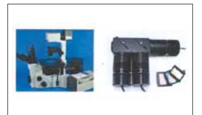
Support for the modification of LED lamp for a inverted microscope installed at a SME
